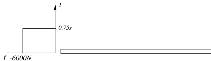
Fig. 5. Loading applied on the end of one-dimensional elastic rod.
