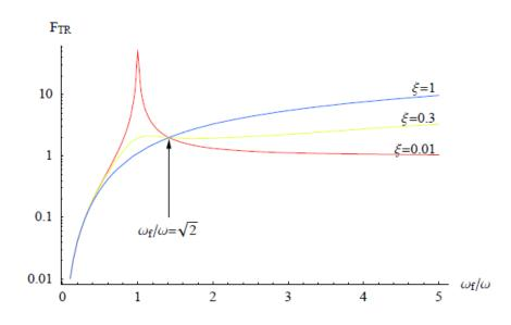
• When the frequency ratio is greater than sqrt(2), the force transmitted is still larger than the static force. It is unlike the displacement transmissibility.
