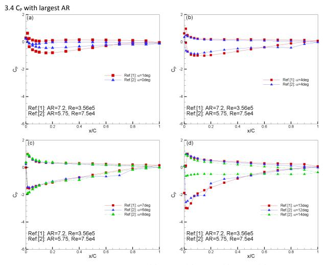
Fig. 14 C<sub>P</sub> distribution with largest AR: (a)  $\alpha \approx 0$  deg, (b)  $\alpha \approx 4$  deg, (c)  $\alpha \approx 7$  deg, (d)  $\alpha \approx 13$  deg
