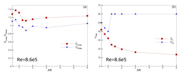
Fig. 9 Aspect ratio dependency of  $C_{Lmax}$  and  $\alpha_{max}$  for  $C_{L}$  in Reference [4]: (a)  $C_{Lmax}$  vs AR, (b)  $\alpha_{max}$  vs AR
