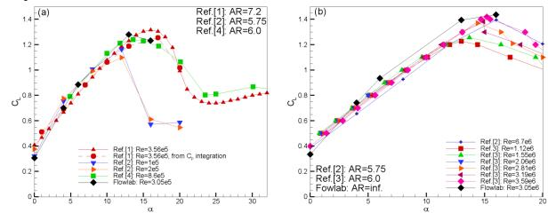
4. Comparison with Flowlab simulation results 4.1  $C_L\,vs\,\alpha$
