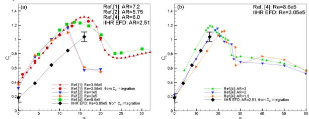
5. Comparison between EFD benchmark data and IIHR experimental data 5.1  $C_L$  vs  $\alpha$
