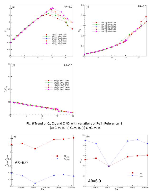
Fig. 7 Re dependency of  $C_{Lmax}$  and  $\alpha_{max}$  for  $C_{L}$  in Reference [3]: (a)  $C_{Lmax}$  vs Re, (b)  $\alpha_{max}$  vs Re
