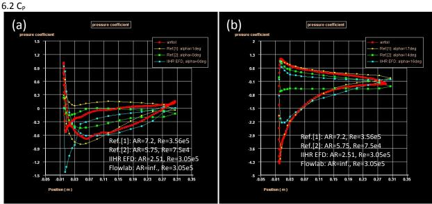
Fig. 23 C<sub>P</sub> distribution: (a)  $\alpha \approx 0$ deg, (b)  $\alpha \approx 16$ deg
