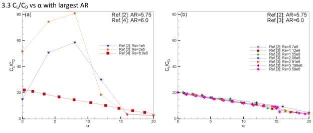
Fig. 12  $C_D$  vs  $\alpha$  with largest AR: (a) Re=O(10<sup>5</sup>), (b) Re=O(10<sup>6</sup>)
