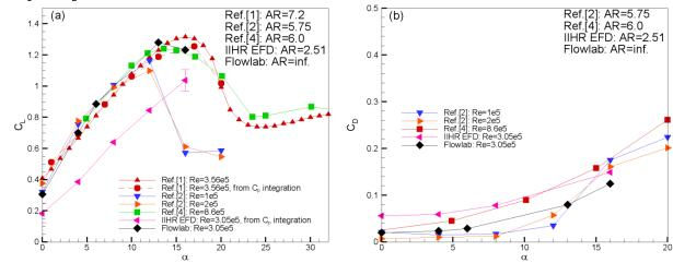
6. Comparison between EFD benchmark data, IIHR experimental data and Flowlab solution 6.1 CL and CD vs  $\alpha$
