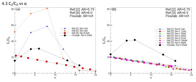
Fig. 17  $C_D$  vs  $\alpha$  with largest AR, Flowlab solutions added: (a) Re=O(10<sup>5</sup>), (b) Re=O(10<sup>6</sup>)
