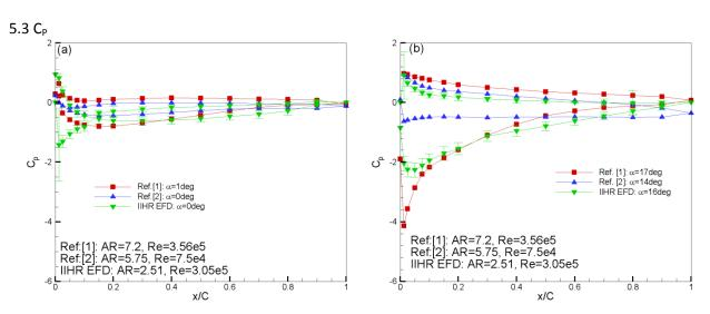
Fig. 21 C<sub>P</sub> distribution, IIHR EFD data added: (a)  $\alpha \approx 0$  deg, (b)  $\alpha \approx 16$  deg
