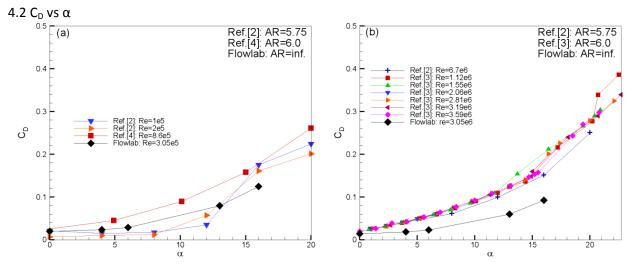
Fig. 16  $C_D$  vs  $\alpha$  with largest AR, Flowlab solutions added: (a) Re=O(10<sup>5</sup>), (b) Re=O(10<sup>6</sup>)
