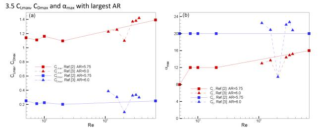
Fig. 13 Re dependency for  $C_{Lmax}$ ,  $C_{Dmax}$  and  $\alpha_{max}$ : (a)  $C_{Lmax}$ ,  $C_{Dmax}$  vs Re, (b)  $\alpha_{max}$  vs Re
