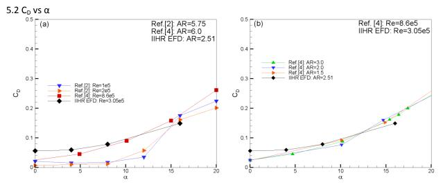
Fig. 20 C<sub>D</sub> vs  $\alpha$ , IIHR EFD data added: (a) large AR ( $\geq$ 5.75), (b) small AR (1.5 $\leq$ AR $\leq$ 3)
