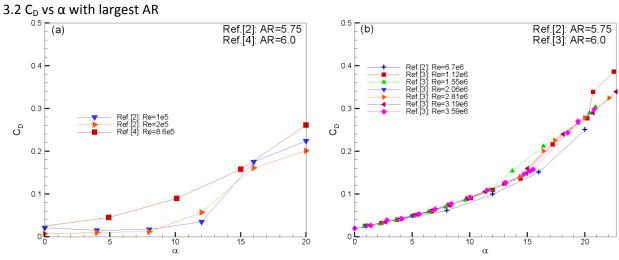
Fig. 11 C<sub>D</sub> vs  $\alpha$  with largest AR: (a) Re=O(10<sup>5</sup>), (b) Re=O(10<sup>6</sup>)
