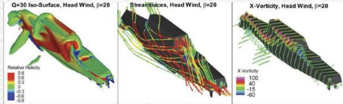
Air flow for ONR Tumblehome in Planar motion mechanism (PMM) maneuvers Movie
