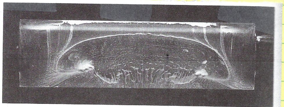
Figure 20.19 Plan view of the trailing-edge stall pattern on a Clark Y-14 airfoil. The pattern is made visible by the oil-flow technique. Flow is from top to bottom. Photography courtesy of A. Winkelmann, Department of Aerospace Engineering, University of Maryland. Reprinted with permission.
