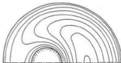
FIGURE 3-9 Constant-velocity lines for an eccentric annulus, b/a = c/a = \frac{1}{2} . [After Fiercy et al. (1933).]
