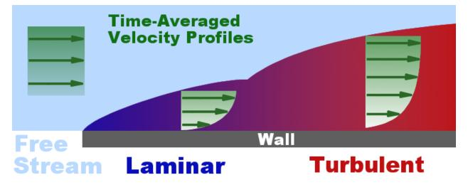
In physics and fluid mechanics, a boundary layer is the layer of fluid in the immediate vicinity of a bounding surface where the effects of viscosity are significant. In the Earth's atmosphere, the atmospheric boundary layer is the air layer near the ground affected by diurnal heat, moisture, or momentum transfer to or from the surface. On an aircraft wing the boundary layer is the part of the flow close to the wing, where viscous forces distort the surrounding non-viscous flow.
