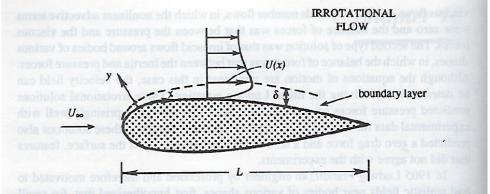
Figure 10.1 The boundary layer. Its thickness is greatly exaggerated in the figure. Here,  $U_{\infty}$  is the oncoming velocity and U is the velocity at the edge of the boundary layer.
