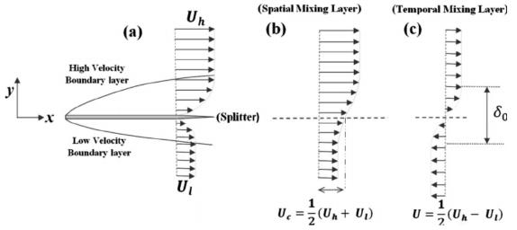
Consider high Re flow (1) around streamlined/slender body for which viscous effects are confined to a narrow boundary layer near the solid surface/wall or (2) for free shear flows, i.e. jets, wakes and mixing layers for which the vorticity is similarly confined to a narrow region. In both cases Prandtl's boundary layer theory is applicable.
