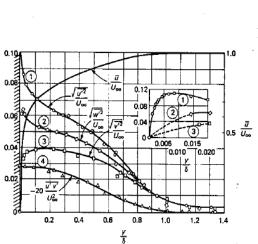
First the best flat the fluctuating velocities u' (streamwise), v' (normal), and w' (lateral) and the turbulent shear u'v'. [After Klebanoff (1955).]
