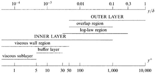
Fig. 7.8. A sketch showing the various wall regions and layers defined in terms of  $y^+ = y/\delta_y$  and  $y/\delta$ , for turbulent channel flow at high Reynolds number (Re<sub>t</sub> = 10<sup>4</sup>).
