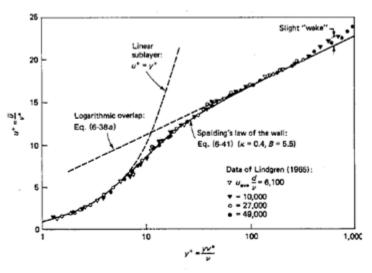
FIGURE 6-11 Comparison of Spalding's inner-law expression with the pipe-flow data of Lindgren (1965).
