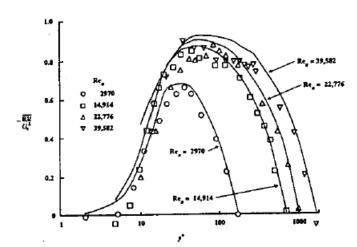
Fig 31. Reynolds stress profiles non-dimensionalized on inner variables. Channel flow data of Wei and Willmarth (1989) at four different Reynolds numbers. Solid line represents momentum balance calculations.
