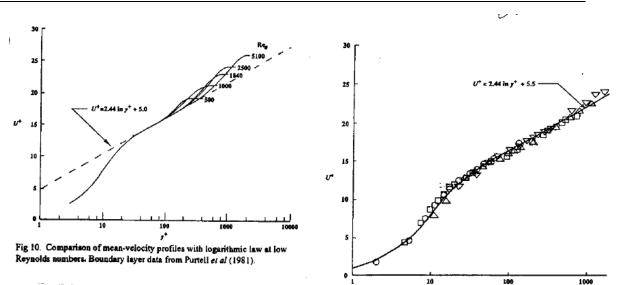
Fig 12. Mean-velocity profiles non-dimensionalized on inner variables. Channel flow data from Wei and Willmarth (1989).
