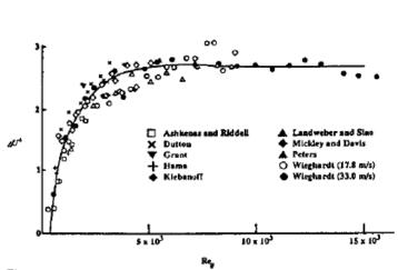
Fig 13. Reproduction of Coles' (1962) strength of the wake component in equilibrium turbulent boundary layers at low Reynolds numbers.
