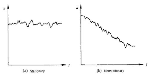
Fig. 12.2 Stationary and nonstationary time series.
