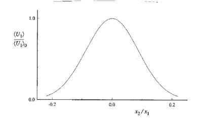
Fig. 1.4. The mean axial velocity profile in a turbulent jet. The mean velocity  $\langle U_1 \rangle$  is normalized by its value on the centerline,  $\langle U_1 \rangle_0$ ; and the cross-stream (radial) coordinate  $x_2$  is normalized by the distance from the nozzle  $x_1$ . The Reynolds number is 95,500. Adapted from Hussein, Capp, and George (1994).
