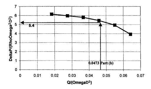
(b) The dimensionless chart above is valid for the new conditions, also. Convert 400 gal/min to 0.891 ft<sup>3</sup>/s and  $\Omega = 900$  rev/min to 15 rev/s. Then evaluate  $\Pi 2$ :
