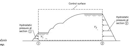
FIGURE 15.18 Control-volume analysis for the hydraulic jump.
