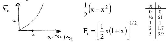
For this particular application we can determine the functional relationship through the use of a control volume analysis: (neglecting  $\mu$  and bottom friction) x-momentum equation:  $\sum F_x = \sum V_x \rho \underline{V} \cdot \underline{A}$
