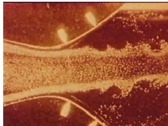
Separations on airfoil (different attack angles)
