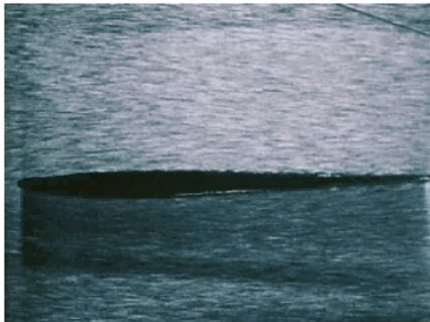
Effect of body shape on separation
