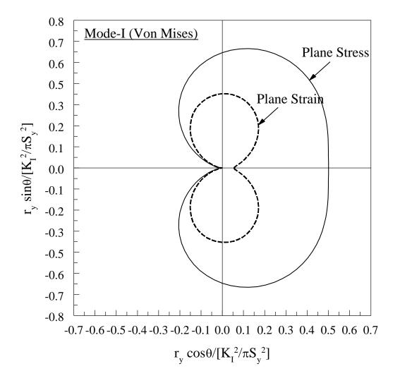
**Comment:** Plastic zone from von Mises yield criterion in plane strain is significantly smaller than that in plane strain.
