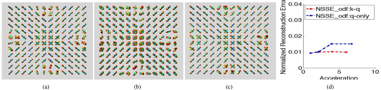
**Fig. 2.** Numerical phantom results: (a) Reference ODF reconstructed using 47 angular measurements. (b),(c) ODF reconstructed at acceleration of 4 using q-only and k-q down-sampling respectively. (d) Plot of Normalized reconstructed error for ODF for the two schemes at various accelerations .
