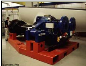
1.5 MW turbine gearbox
