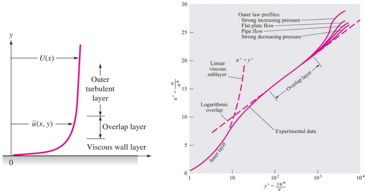
Turbulent flat-plate flow is nearly logarithmic, with a slight outer wake and a thin viscous sublayer,
