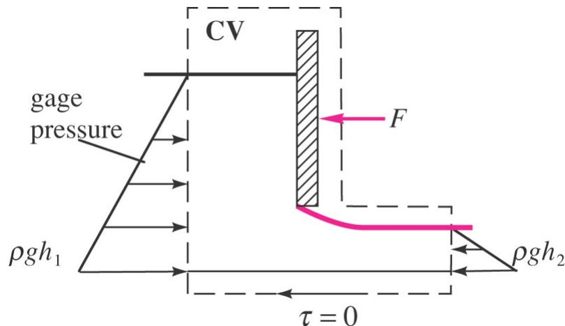
Assume steady incompressible flow with no variation across the width  $b$ . The inlet and outlet mass flows balance:
