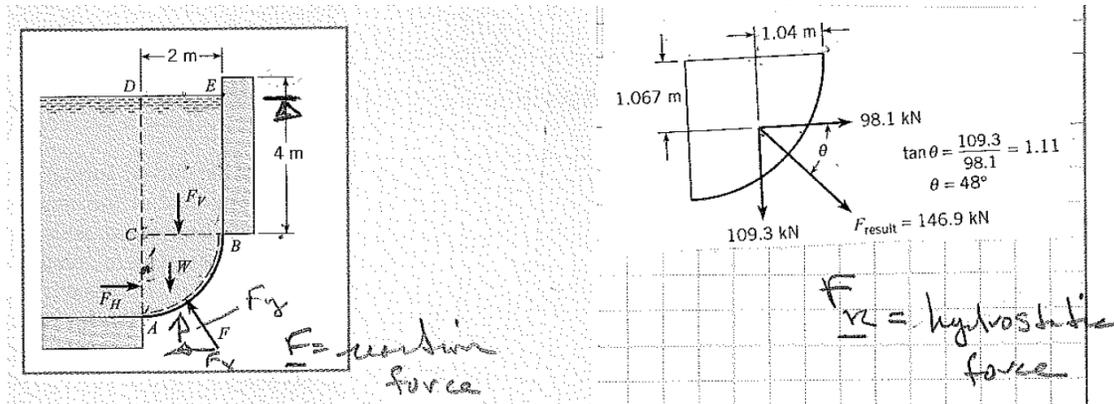
In the figure, surface  $AB$  is a circular arc with a radius of 2m and a depth of 1m into the paper. The distance  $EB$  is 4m. The fluid above surface  $AB$  is water, and atmospheric pressure prevails on the free surface of the water and on the bottom side of surface  $AB$ . Find the magnitude and line of action of the hydrostatic force acting on surface  $AB$ .
