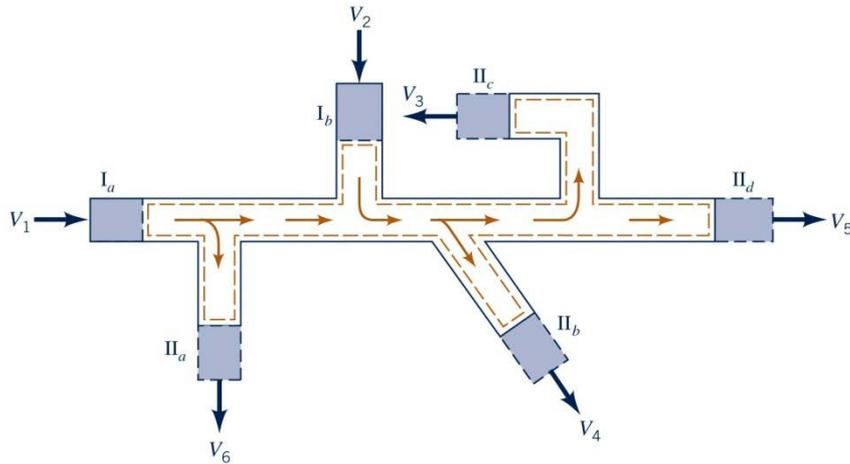
Typical control volume with more than one inlet and outlet.
