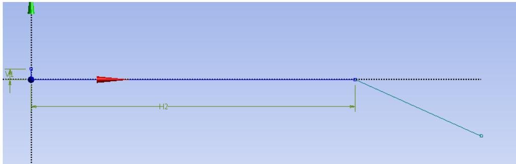
4.10 Sketching > Dimensions > Angle. Select the line circled in red below then select the x-axis then change the angle to 10 degrees.
