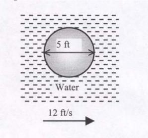
The density of water:  $62.41 \text{ bm/ft}^3$ . Drag coefficient for a sphere:  $C_D = 0.2$  for turbulent flow  $C_D = 0.5$  for laminar flow
