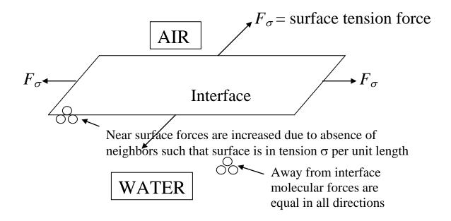
$\sigma_{\text{air/water}} = 0.073 \text{ N/m}$   $F_{\sigma} = \sigma \times L = \text{line force with direction normal to the cut}$  L = length of cut through the interface
