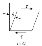
No slip condition: no relative motion between fluid and boundary, i.e., fluid in contact with lower plate is stationary, whereas fluid in contact with upper plate moves at speed *U*.
