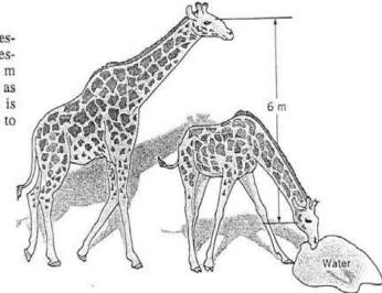
(a) For hydrostatic pressure change,  $\Delta p = 8 - h = \left(9.80 \frac{kN}{m^2}\right) (6 \text{ m}) = 58.8 \frac{kN}{m^2} = \frac{58.8 \text{ kfa}}{8.8 \text{ m}} = \frac{58.8 \text{ kfa}}{10.8 \text{$
