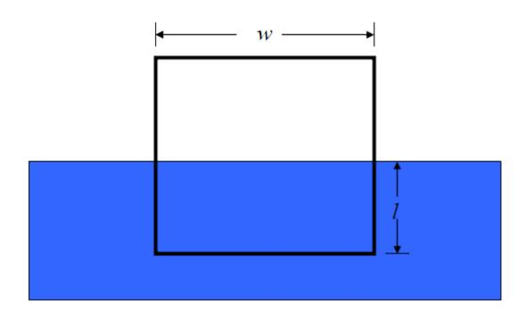
**Solution:** For neutral stability, the distance to the metacenter is zero.
