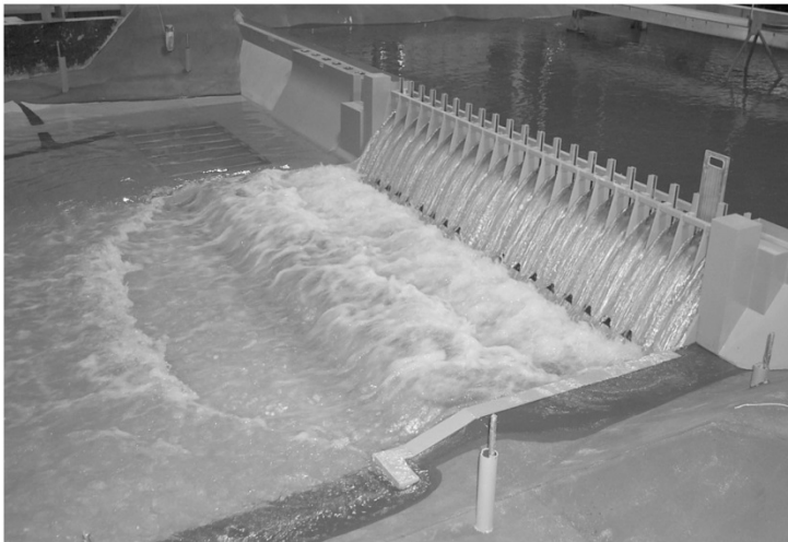
Fig. 5.9 Hydraulic model of the Bluestone Lake Dam on the New River near Hinton, West Virginia. The model scale is 1:65 both vertically and horizontally, and the Reynolds number, though far below the prototype value, is set high enough for the flow to be turbulent. (Courtesy of the U.S. Army Corps of Engineers Waterways Experiment Station.)
