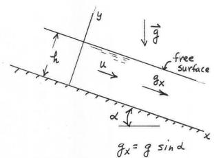
With the coordinate system shown in the figure v=0, w=0, and from the continuity equation  $\frac{\partial u}{\partial x}=0$ . Thus, from the x-component of the Navier-Stokes equations (Eg. 6.127a)
