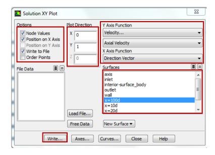
Name the file *CFD Lab 1 Developed Axial Velocity Profile* and leave the **Files of Type:** as XY Files.
