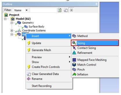
5.6. Hold **Ctrl** button and select the top and bottom edge then click **Apply**. Specify details of sizing as per below in the **Details of "Edge Sizing"** – **Sizing** window.
