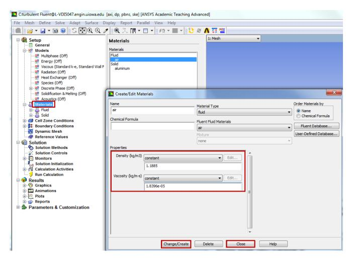
If the room temperature is 24°, the density and viscosity are the values shown in the above panel. **NOTE:** viscosity used in ANSYS is the **dynamic viscosity** ( $kg/m \cdot s$ ), **NOT kinematic viscosity** ( $m^2/s$ )
