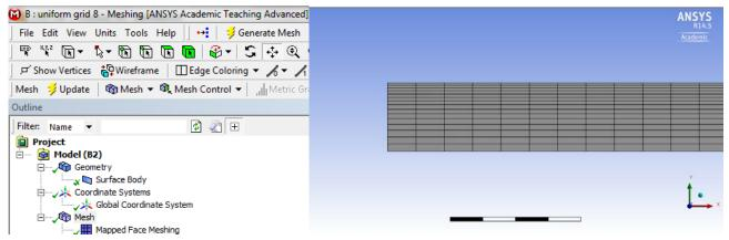
5.10. Change the edge names by selecting the edge, then right clicking on the edge and selecting **Create Named Selection** from the drop down menu. Name left, right, bottom and top edges as *inlet*, *outlet*, *axis* and *wall* respectively then click **OK**. Your outline should look same as the figure below.
