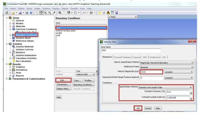
6.9. **Setup** > **Boundary Conditions** > **outlet** > **Edit...** Change gauge pressure as per experimental data. Change other parameters as below and click OK. You need to transform the four pressure tap pressure values from "feet water" to "Pascal" and input pressure tap #4 value as the "outlet pressure". For example, if the pressure tap #4 has value of 0.2502 feet water, you need input 747 Pascal.
