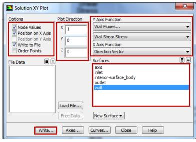
Name the file *CFD Lab 1 Wall Shear Stress Distribution* and leave the **Files of Type**: as XY Files.
