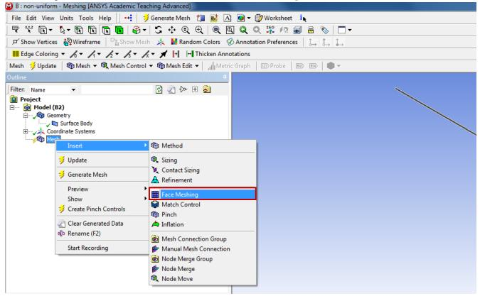
5.3. Select your geometry by clicking on the yellow box which says **No Selection**, then select the geometry surface and click **Apply**. (Note: You can change orientation of your view by clicking the axis figure on the lower right corner. Press "F7" on your keyboard to restore to the "whole view". Zoom in by holding the right mouse button and selecting a region.)
