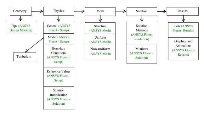
Flow chart for "CFD Process" for pipe flow
