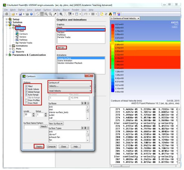
Save the picture as you did for the mesh and call it CFD Lab 1 Contours of Axial Velocity and save it in the folder you created.
