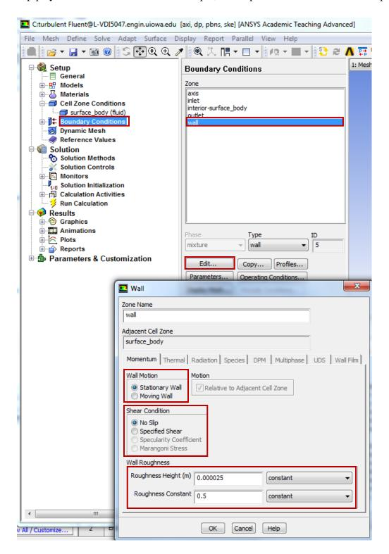
6.11. **Setup > Boundary Conditions > Operating Condition**. Change parameters as per below and click **OK**.
