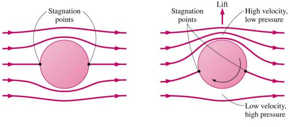
(a) Potential flow over a stationary cylinder
