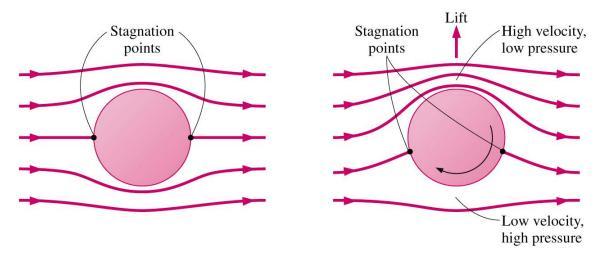
(a) Potential flow over a stationary cylinder
