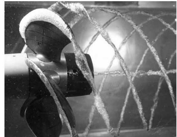
Cavitation formed on a marine propeller
