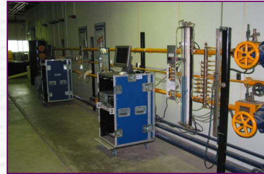
Lab2: Measurement of flow rate, friction factor and velocity profiles in smooth and rough pipes, and measurement of flow rate through a nozzle using PIV technique.
