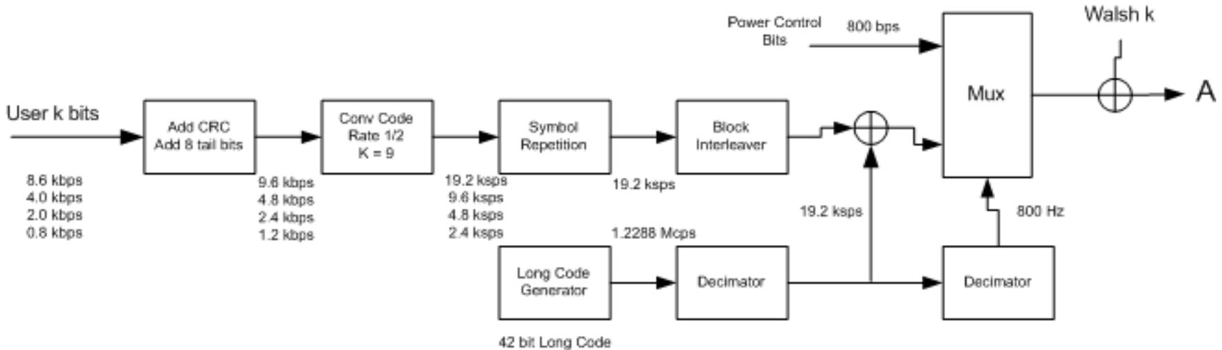
This transmitter structure is used in the base station by Sprint PCS, Verizon, and worldwide
