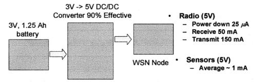
WSN node is programmed to turn on radio every 5 seconds, listen on the network for 0.5 seconds, and then power down the radio.
