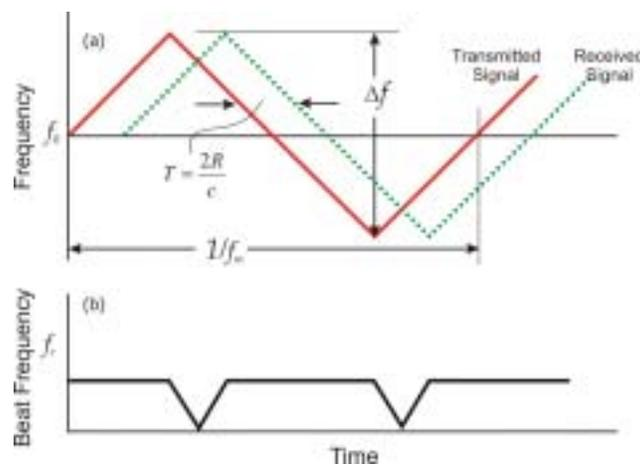
In the figure, (a) is the frequency-time relationship of an FM-CW radar with triangular modulation. The received signal (dashed line) from a target at range  $R$  is delayed a time  $T = \frac{2R}{c}$ .  $\Delta f$  is the frequency excursion and  $f_m$  is the modulation frequency. In (b) is the difference (beat) frequency between the transmitted and received signals. One can show that for a stationary target:
