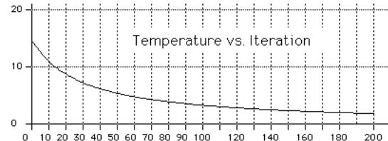
$$T_{i+1} = \frac{T_i}{1 + \beta T_i} \quad \text{where} \quad \beta = \frac{(T_0 - T_f)}{M T_0 T_f} \quad \& \quad \begin{cases} T_0 = \text{initial temperature} \\ T_f = \text{final temperature} \\ M = \# \text{ of iterations} \end{cases}$$
