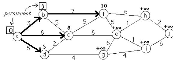
Next step is to choose the temporary label to be made permanent. This will be the label of node d, which is the smallest temporary label.
