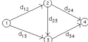
Example: Find the shortest path from node  $1$  to node  $4$ , where distances are as given.
