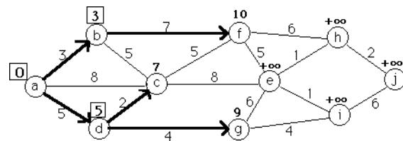
The next temporary label to be made permanent is that of node c.
