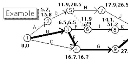
Using  $\mu$  as the duration of each activity, find the critical path.
