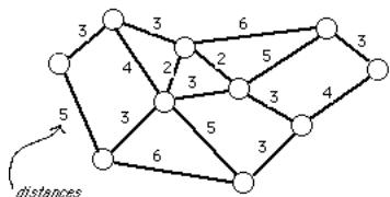
Where on the network should one locate an emergency facility (for example, a fire station) so as to minimize the distance to the furthest node in the network?
