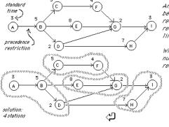
An assembly line is to be designed for a job requiring 9 tasks. The required output of the line is 6/hour.
