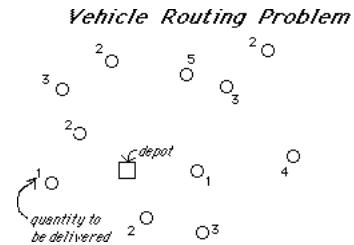
Delivery trucks with a capacity of 8 units are to deliver to customers. What is the lowest cost set of routes? (Assume fixed cost of using truck, plus cost proportional to distance.)
