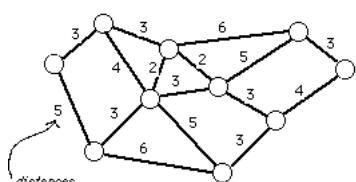
Given a set of facilities and a network representing possible links to be built, what is the set of links with least distance such that every facility can communicate with each of the other facilities?
