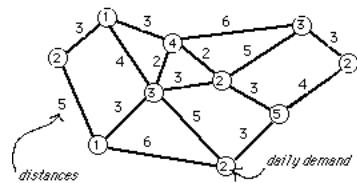
Where on the network should one locate two facilities so as to minimize the daily cost of satisfying the demands? (assuming costs are linear in both distance and quantities shipped)
