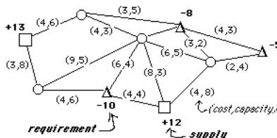
What is the lowest-cost way to ship supplies of goods from supply points to demand points, given a network with specified shipping cost/unit and capacity in each link?
