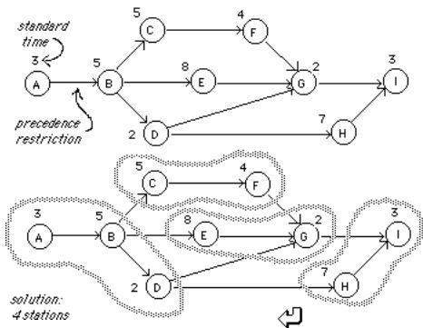
An assembly line is to be designed for a job requiring 9 tasks. The required output of the line is 6/hour.
