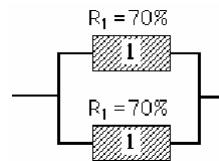
The reliability of a component may be increased by including redundant units!
