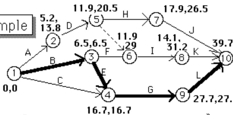
Using  $\mu$  as the duration of each activity, find the critical path.
