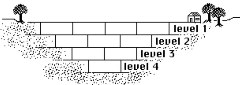
Restrictions imposed by the angle of slip means that it is possible only to excavate blocks forming an "inverted pyramid"
