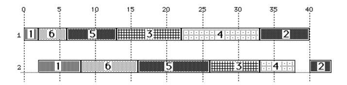
3-Machine Flow Shop Special conditions under which Johnson's Algorithm can be used to minimize the makespan:
