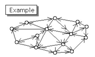
The nodes on a path through the network correspond to a sequence of products which can be produced with a single major setup.
