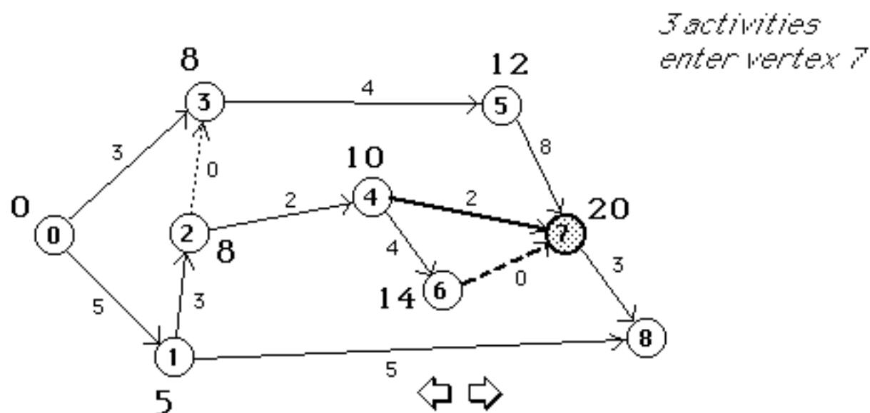
$$\begin{aligned} ET(8) &= \max\{ET(1)+5, ET(7)+3\} \\ &= \max\{10, 23\} = 23 \end{aligned}$$
