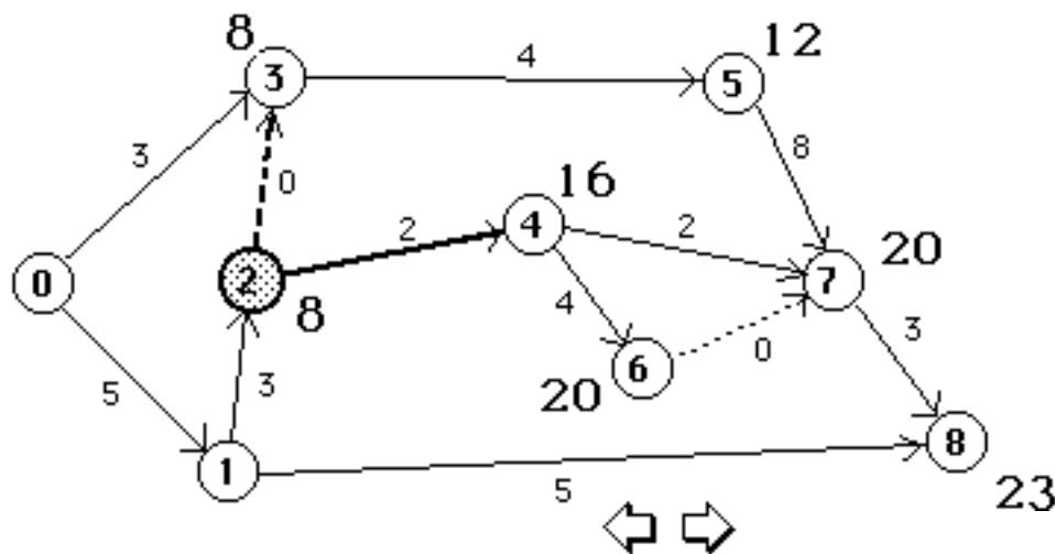
$$\begin{aligned} LT(1) &= \min\{LT(2)-3, LT(8)-5\} \\ &= \min\{5, 18\} = 5 \end{aligned}$$
