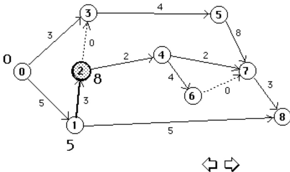
$$\begin{aligned} ET(3) &= \max(ET(0)+3, ET(2)+0) \\ &= \max\{3,8\} = 8 \end{aligned}$$
