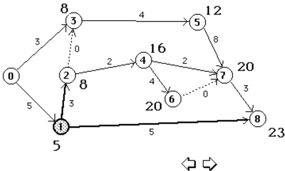
$$\begin{aligned} LT(0) &= \min\{LT(1)-5, LT(3)-3\} \\ &= \min\{0, 5\} = 0 \end{aligned}$$
