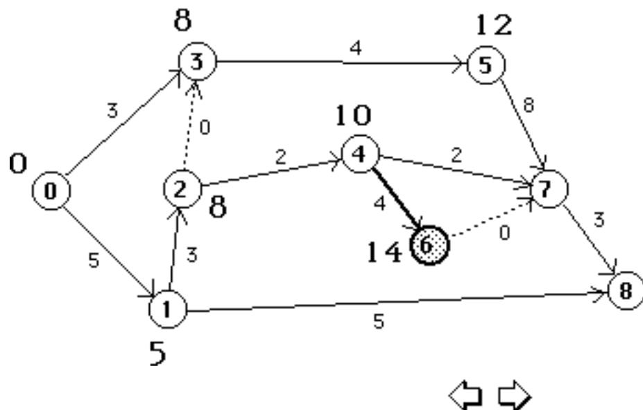
$$\begin{aligned} ET(7) &= \max\{ET(4)+2, ET(6)+0, ET(5)+8\} \\ &= \max\{12, 14, 20\} = 20 \end{aligned}$$
