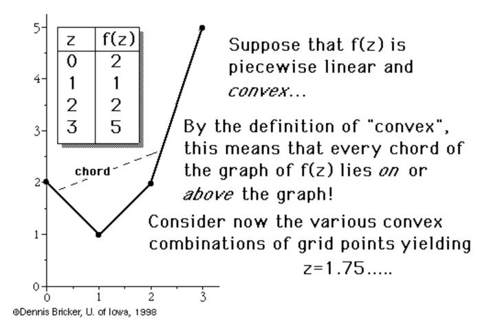
A given value of z, e.g., z=1.75, can be represented by several different convex combinations of the grid points:
