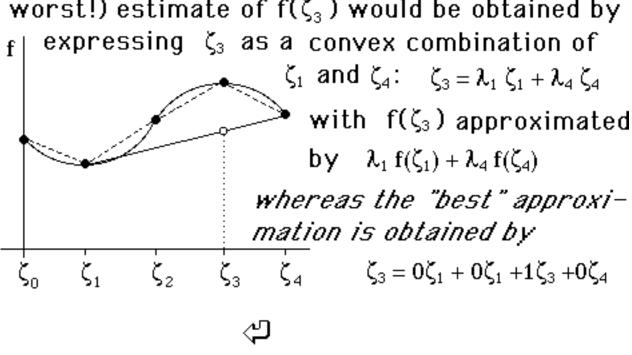
In the "lambda" formulation, a special variable ( $\lambda$ ) was defined for each grid point. In the "delta" formulation, a special variable ( $\delta$ ) will be defined for each interval between grid points, i.e., for each linear piece.
