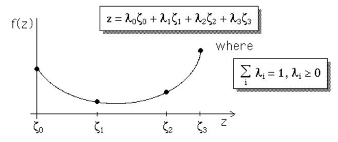
With the same "weights" used in writing the convex combination of the grid points,
