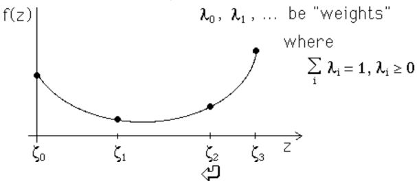
Any value of z in the interval between the left-most and the right-most grid point may be expressed as a "convex combination" of the grid points:
