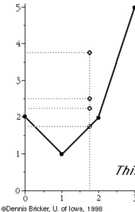
Of the various ways to express z as a convex combination of grid points, the way which results in the *minimum* value for an approximation of f(z)is that which assigns positive weights only to the grid points immediately to the left and right of z.
