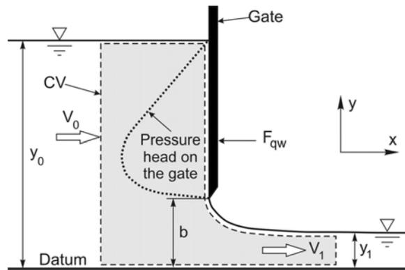
Figure 1. Flow under a vertical sluice gate.
