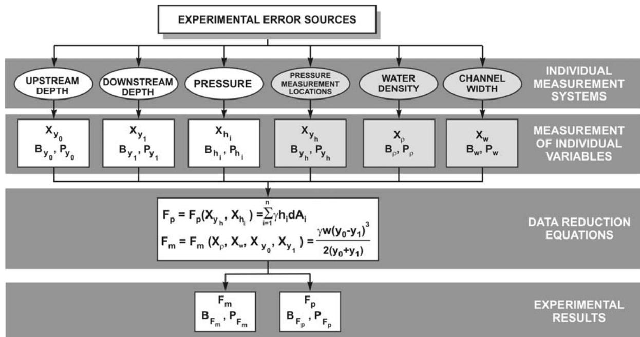
Figure 3. Block Diagram of the sluice gate experiment including measurement systems / data reduction equations
