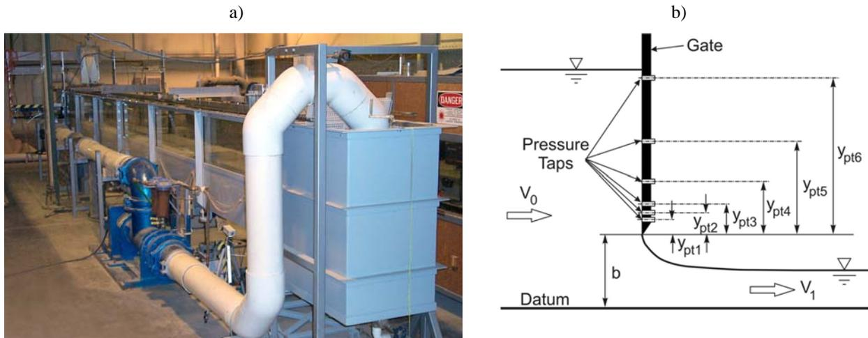
Figure 2. Experimental setup: a) the experimental flume; b) positioning of the pressure taps onto the sluice gate
