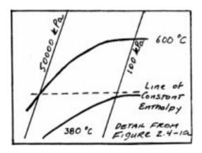
For the ideal gas, enthalpy is a function of temperature only. Thus,  $\underline{H}(T_1, P_1) = \underline{H}(T_2, P_2)$  becomes  $\underline{H}(T_1) = \underline{H}(T_2)$ , which implies that  $T_1 = T_2 = 600^{\circ} \mathrm{C}$ .
