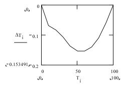
The temperature error plotted here results from the nonlinear dependence of the volume of mercury on temperature. In a real thermometer there will also be an error associated with the imperfect bore of the capillary tube.
