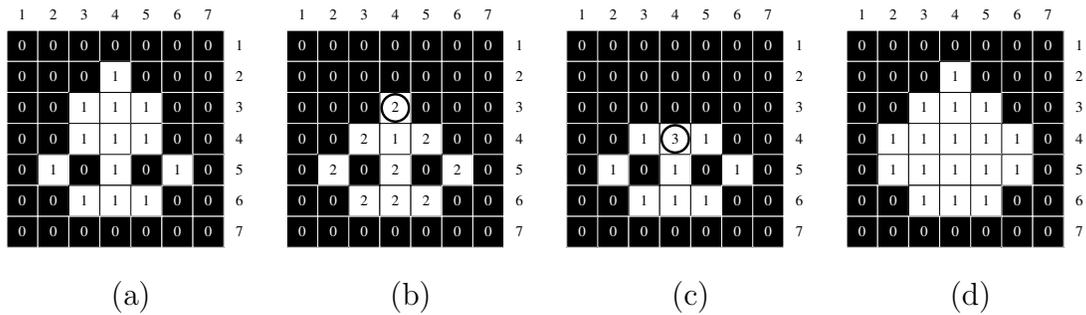
Fig. 5. (a): Original image. (b): Intermediate result after the first thinning step, with contour pixels labeled 2. (c): Final skeleton with labels. (d): Reconstructed object.
