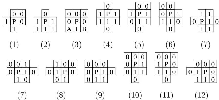
Fig. 13. Masks for the Choy, Choy and Siu's algorithm. (1, 2, 3): thinning masks (with all their  $\pi/2$  rotations). (4, 5, 6, 7, 8, 9, 10, 11, 12): restoring masks. For mask 3, at least one of the pixels  $A, B$  must be in  $X$ .
