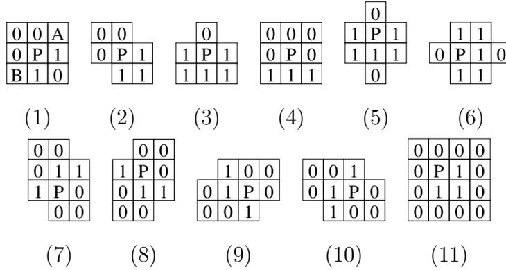
Fig. 12. Masks for the Jang and Chin's JC93 algorithm. (1, 2, 3, 4): thinning masks (with all their  $\pi/2$  rotations). (5, 6, 7, 8, 9, 10, 11): restoring masks. For mask 1, at least one of the pixels  $A, B$  must be in  $X$ .
