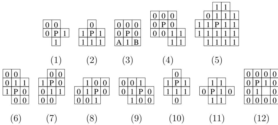
Fig. 10. Masks for the Jang and Chin’s JC92 algorithm. (1, 2, 3, 4, 5): thinning masks (with all their  $\pi/2$  rotations). (6, 7, 8, 9, 10, 11, 12): restoring masks (12 with all its  $\pi/2$  rotations). For mask 3, at least one of the pixels  $A, B$  must be in  $X$ .
