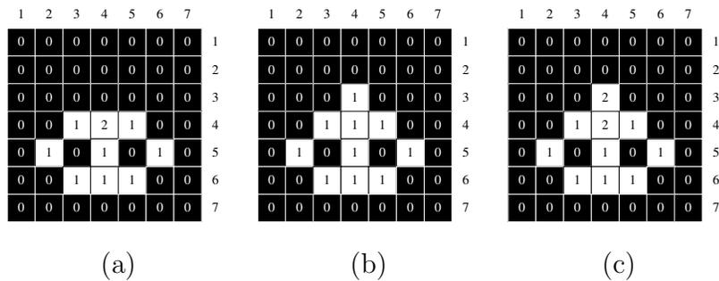
Fig. 6. (a): Skeleton with pixels labeled by their distance to the background. (b): Object reconstructed from (a). (c): Correct labeled skeleton allowing exact reconstruction.
