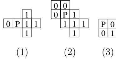
Fig. 15. Masks for the Bernard and Manzanera’s algorithm. (1, 2): thinning masks (with all their  $\pi/2$  rotations). (3): restoring mask (with all its  $\pi/2$  rotations).
