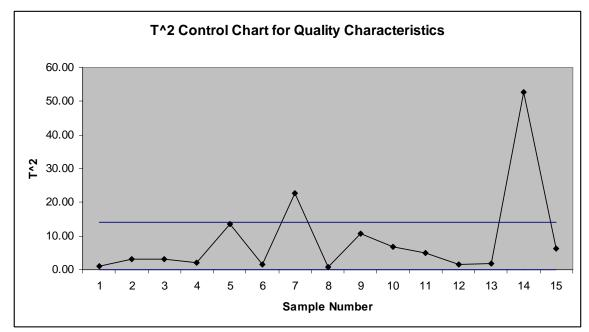
Process is out of control at samples 7 and 14.
