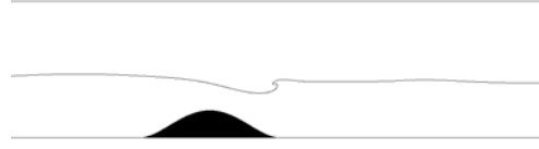
Figure 22. Computational domain for breaking waves over a surface-mounted bump.
